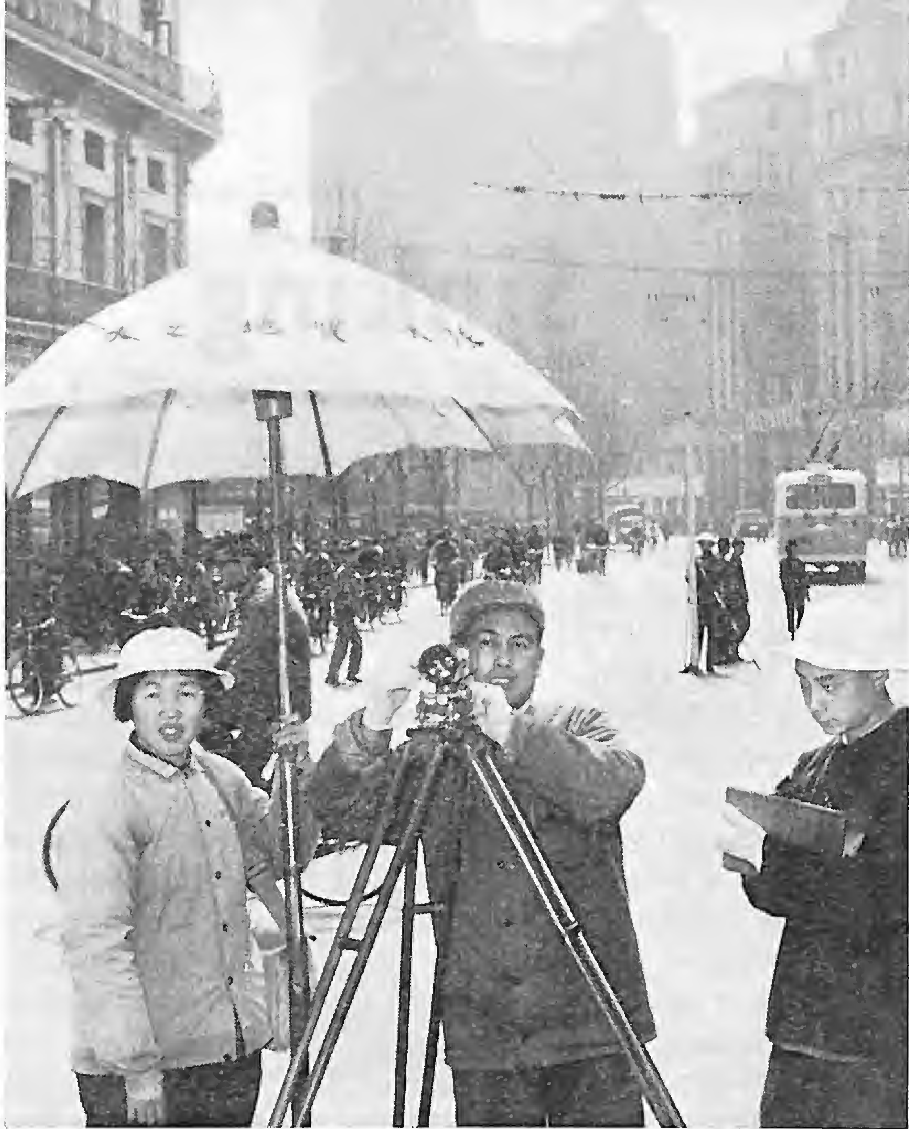
The rise in Shanghai's land after measures were taken to control sinking is checked by members of the Shanghai Hydrogeological Survey Team.
